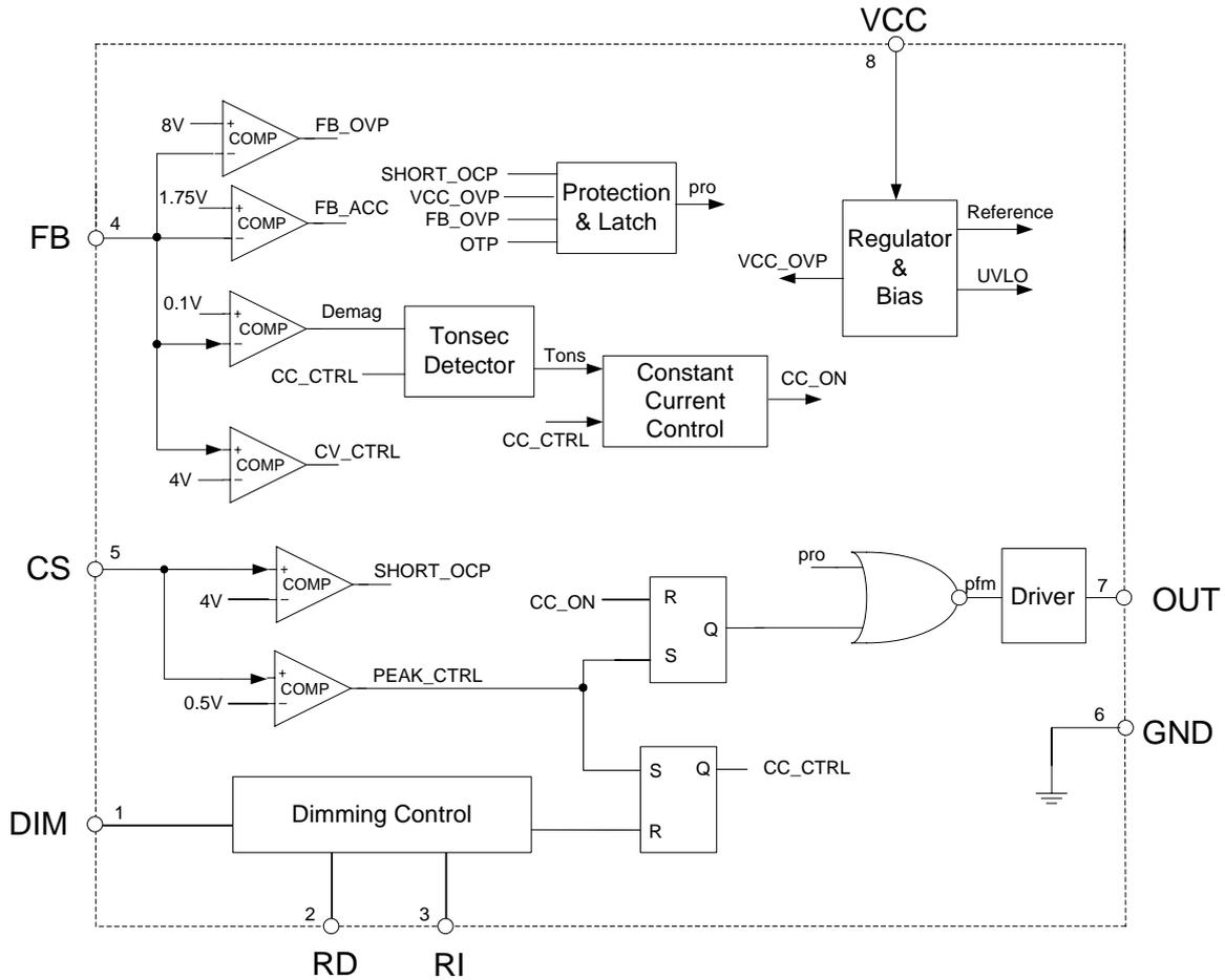
Figure 3. Functional Block Diagram of AP1681
