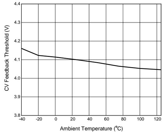
Figure 11. CV Feedback Threshold vs. Ambient Temperature
