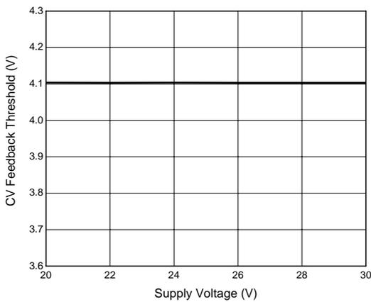
Figure 12. CV Feedback Threshold vs. Supply Voltage
