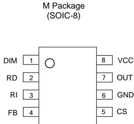
Figure 2. Pin Configuration of AP1681 (Top View)
