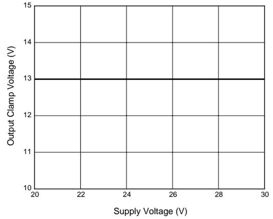
Figure 15. Output Clamp Voltage vs. Supply Voltage
