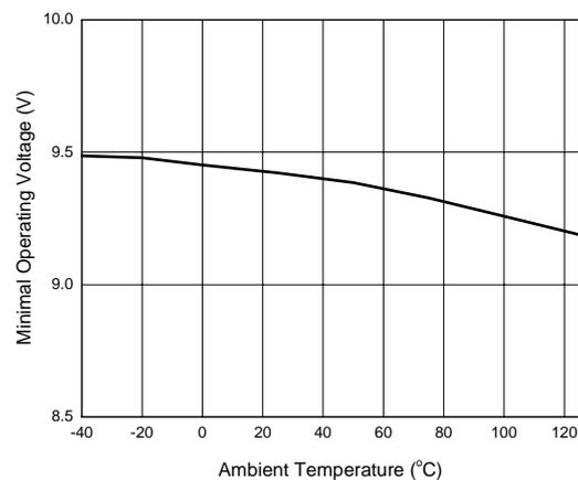
Figure 5. Minimal Operating Voltage vs. Ambient Temperature
