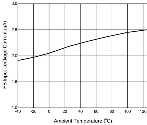
Figure 14. FB Input Leakage Current vs. Ambient Temperature
