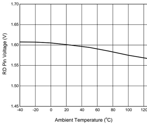
Figure 16. RD Pin Voltage vs. Ambient Temperature
