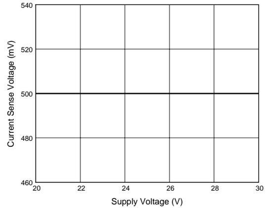
Figure 9. Current Sense Voltage vs. Supply Voltage
