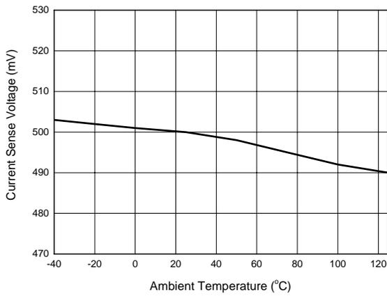
Figure 10. Current Sense Voltage vs. Ambient Temperature
