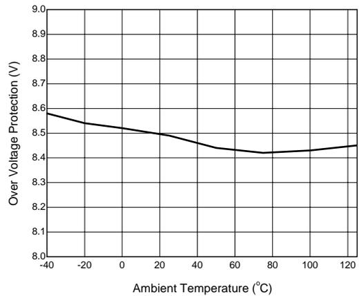
Figure 13. Over Voltage Protection vs. Ambient Temperature
