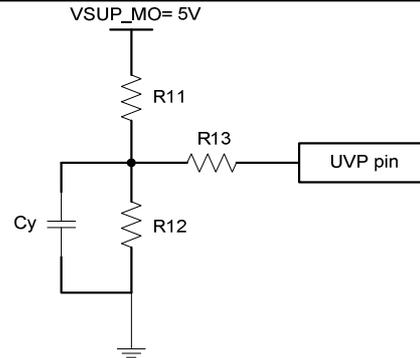
To minimize the system power-up and power-down threshold variations, resistors with less than 1% variations are recommended. Although some resistor value options are offered above for customer's reference or starting points, customers should always verify those resistor options in their actual design. Customer can adjust their own design to achieving the best performance between pop noise and power-on threshold by adjusting the passive resistors R11, R12 and R13.
