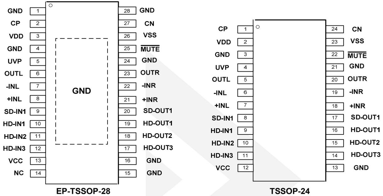
Figure 1 Pin Assignment
