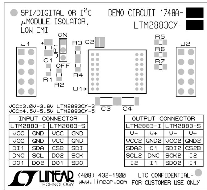
Figure 14a. LTM2883 Low EMI Demo Board Layout
