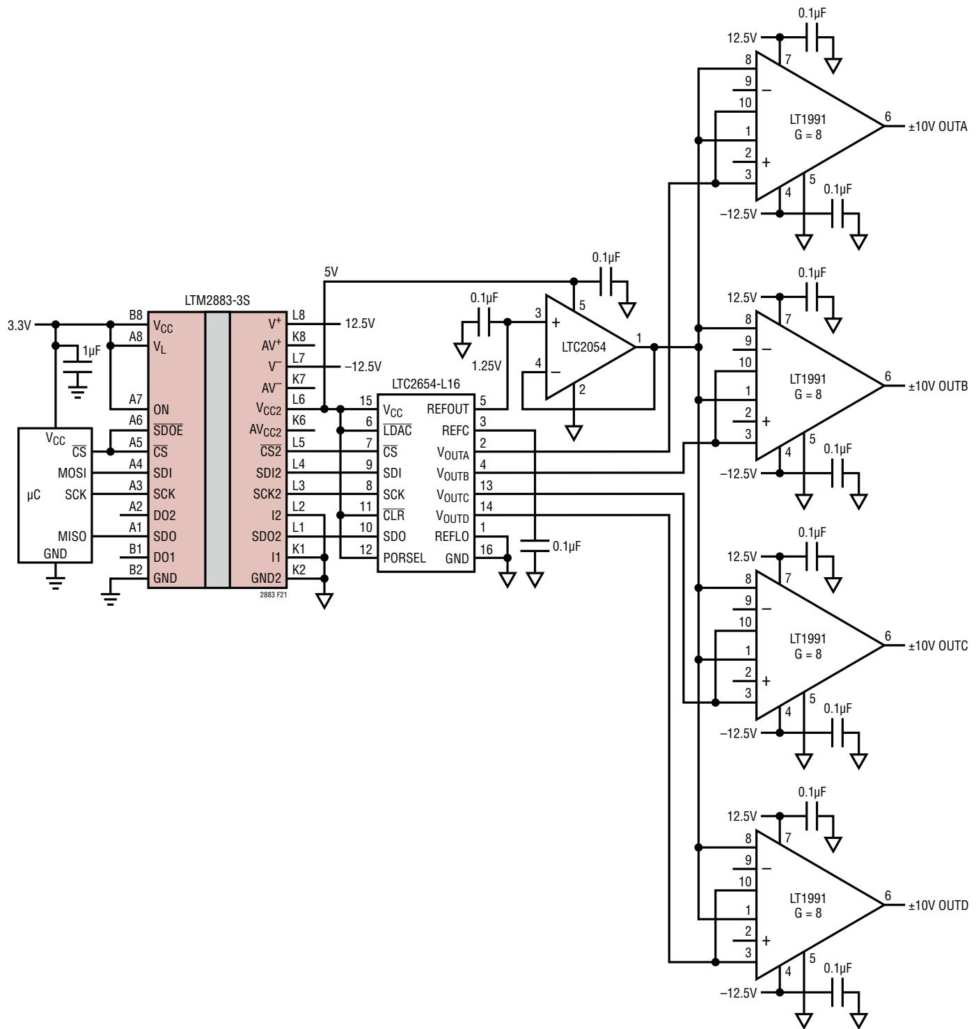
Figure 21. Quad 16-Bit  $\pm 10V$  Output Range DAC
