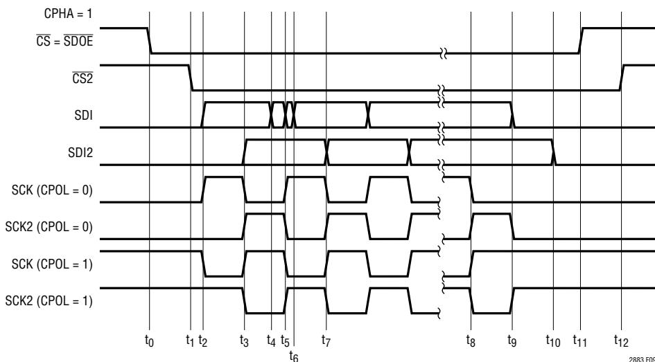
Figure 9. SPI Timing, Unidirectional, CPHA = 1
