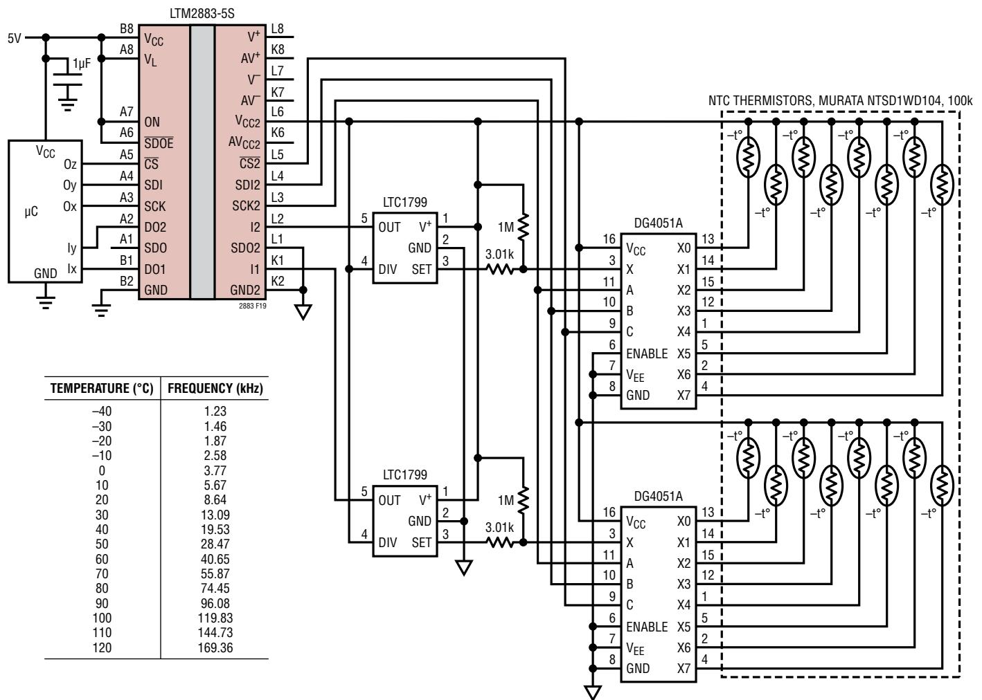
Figure 19. 16-Channel Isolated Temperature to Frequency Converter
