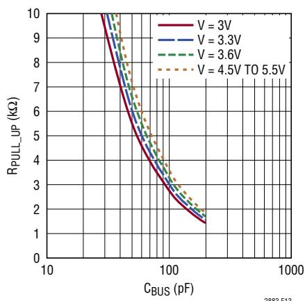
**Figure 13. Maximum Fast Speed Pull-Up Resistance on SDA**
