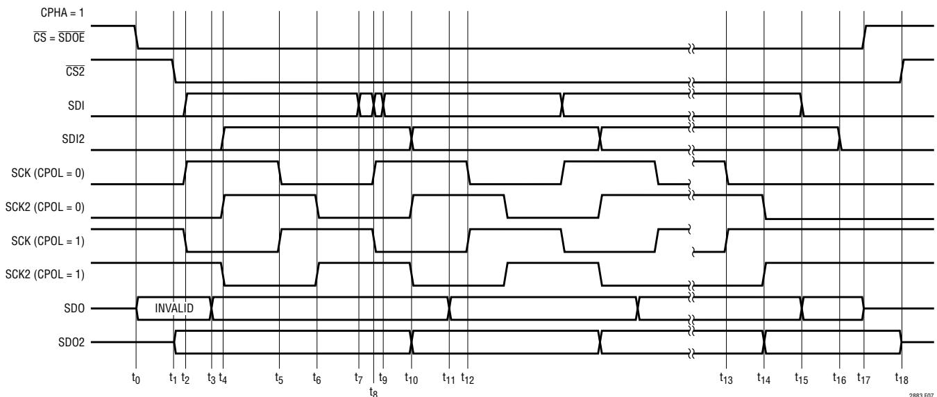
Figure 7. SPI Timing, Bidirectional, CPHA = 1
