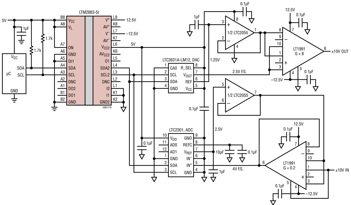
Figure 16. Isolated I<sup>2</sup>C 12-Bit, ±10V Analog Input and Output
