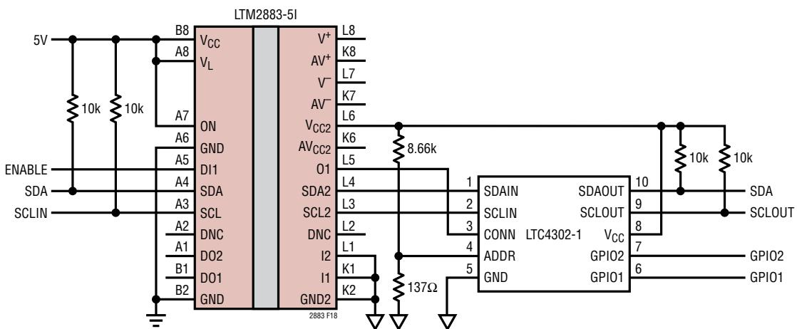
Figure 18. Isolated I<sup>2</sup>C Buffer with Programmable Outputs
