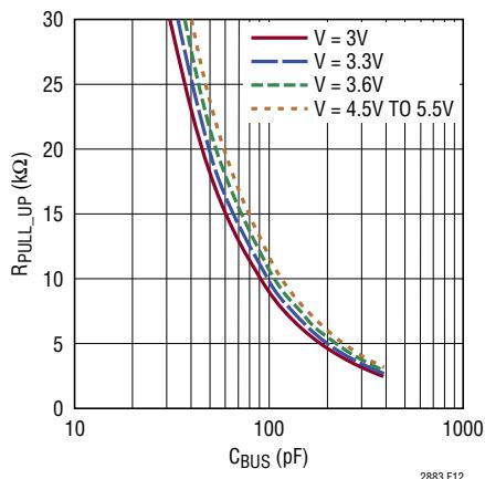
**Figure 12. Maximum Standard Speed Pull-Up Resistance on SDA**
