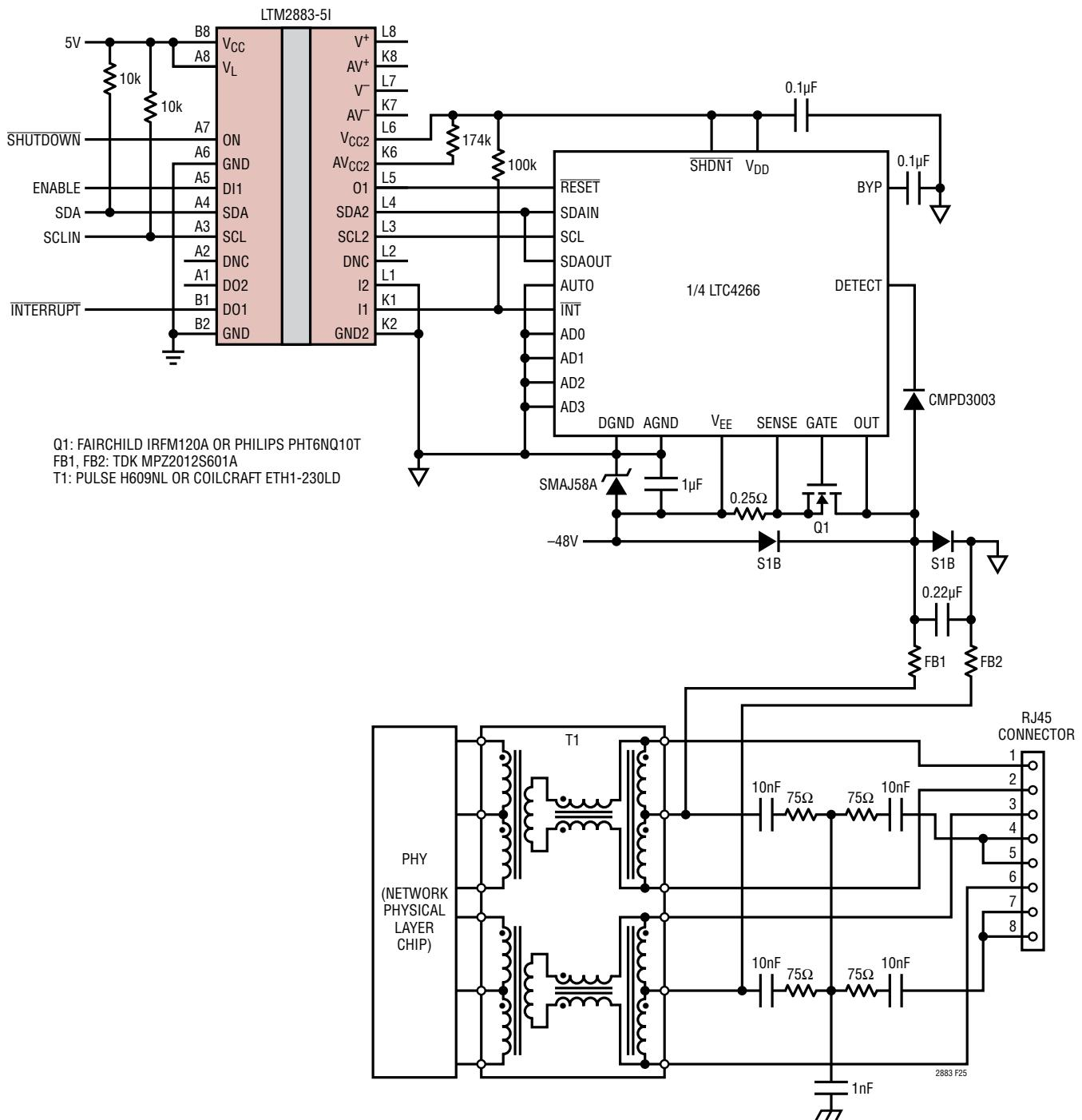
Figure 25. One Complete Isolated Powered Ethernet Port
