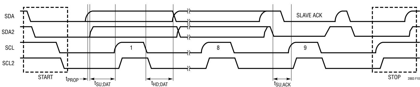
Figure 10. I<sup>2</sup>C Timing Diagram
