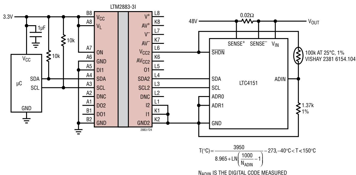
$$T(^{\circ}\text{C}) = \frac{3950}{8.965 + \ln\left(\frac{1000}{N_{ADIN}} - 1\right)} - 273, -40^{\circ}\text{C} < T < 150^{\circ}\text{C}$$
