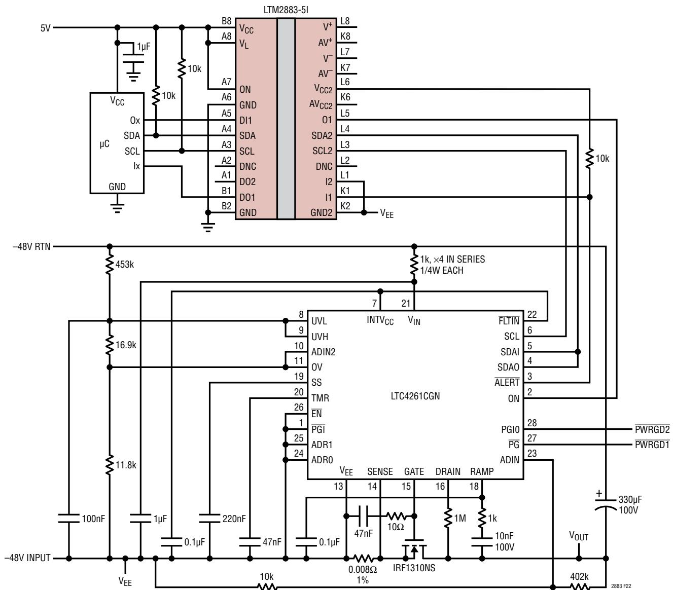
Figure 22. -48V, 200W Hot Swap Controller with Isolated I<sup>2</sup>C Interface
