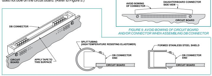
FIGURE 6: THREE TYPICAL MASKING APPLICATIONS FOR SOLDERING DB CONNECTORS
