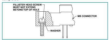
FIGURE 3: MB CONNECTOR WITH SCREW MOUNTING
