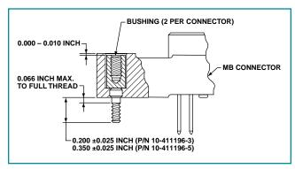
FIGURE 1: ASSEMBLY OF LOCKING/MOUNTING BUSHING INTO MB CONNECTOR
