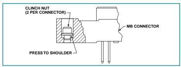
FIGURE 2: MB CONNECTOR WITH CLINCH NUT MOUNTING
