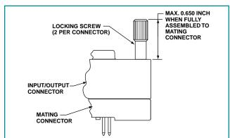
FIGURE 9: I/O LOCKING SCREW DIMENSIONS
