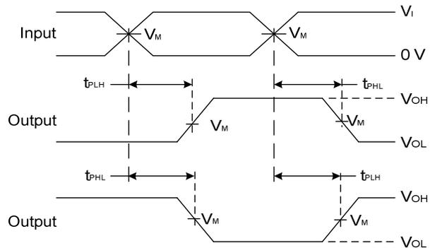
**Voltage Waveform Propagation Delay Times
