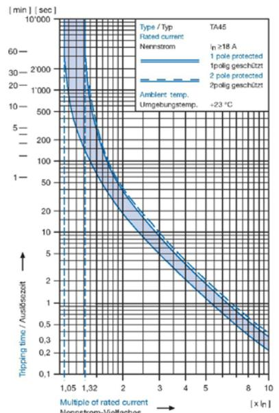
CIRCUIT BREAKERS FOR EQUIPMENT, 2 POLE, ROCKER
