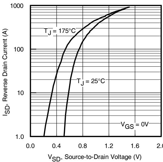
**Fig. 7** Typical Source-to-Drain Diode
