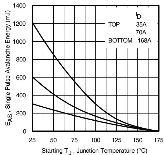
**Fig 12.** Maximum Avalanche Energy vs. Drain Current
