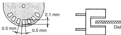
3. The following illustrations show the definition of response delay time. The value in the parentheses applies to the EE-SX4070.
