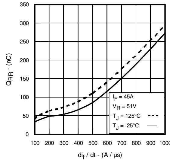
**Fig. 20 -** Typical Stored Charge vs.  $\frac{di}{dt}$
