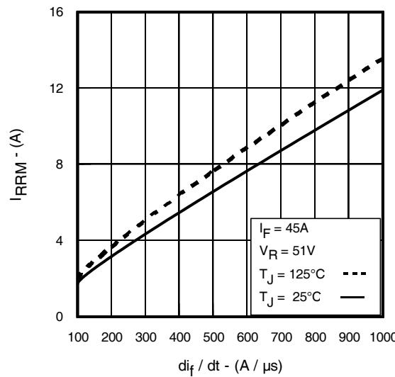
**Fig. 18 -** Typical Recovery Current vs.  $\frac{di}{dt}$
