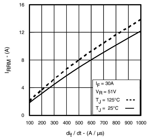
**Fig. 17 -** Typical Recovery Current vs.  $\frac{di}{dt}$
