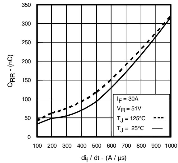
**Fig. 19 -** Typical Stored Charge vs.  $\frac{di}{dt}$
