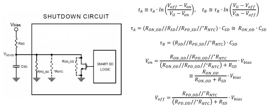
R<sub>SD</sub> and C<sub>SD</sub> external circuitry must be designed to ensure  $V_{on} < V_{il}$  &  $V_{off} > V_{th}$
