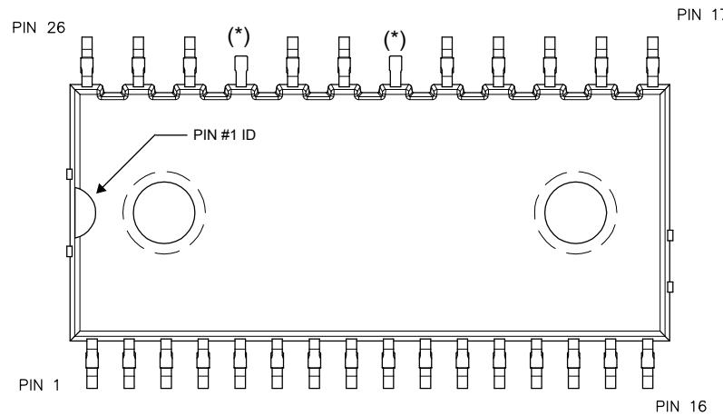
(\*) Dummy pin internally connected to P (positive DC input).
