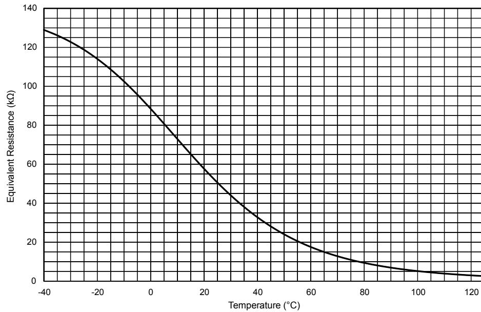
Figure 7. Equivalent resistance (NTC//R<sub>PD\_SD</sub>) zoom
