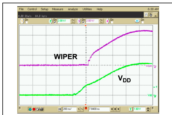
FIGURE 2-15: 2.1 k \Omega – Power-Up Wiper Response Time.
