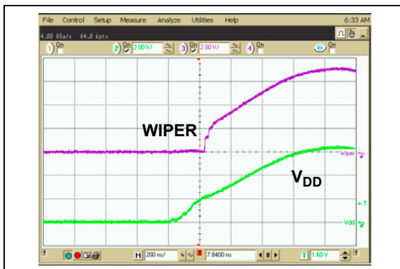
FIGURE 2-52: 50 k \Omega – Power-Up Wiper Response Time.
