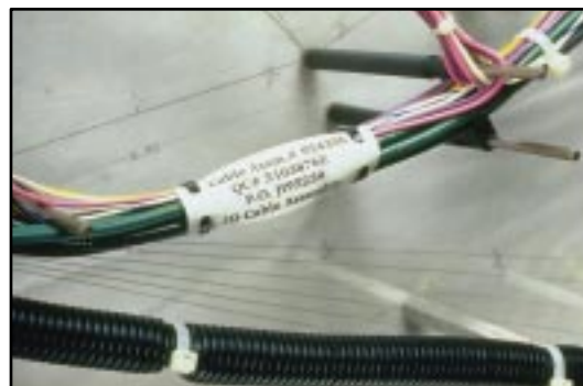
Identify harness board assemblies
