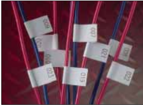
Marking Wires and Cables
