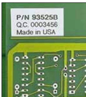
Circuit board labeling
