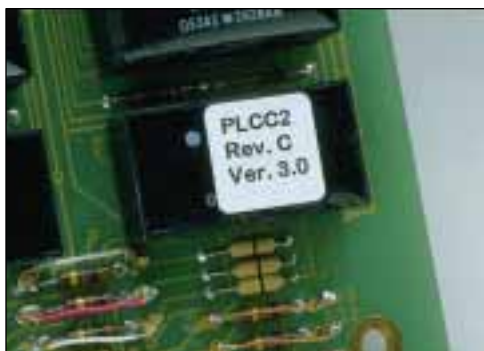
Circuit Board Labeling
