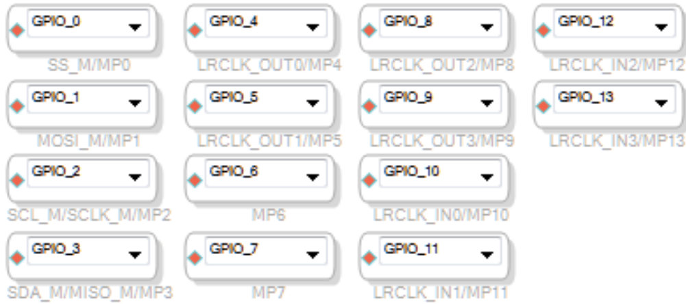
Figure 77. Complete Set of General-Purpose Outputs in SigmaStudio
