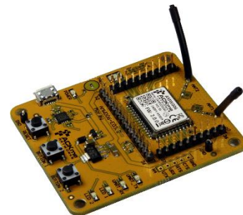
Figure 9 - AMW006-E03 eval board with wire antennas
