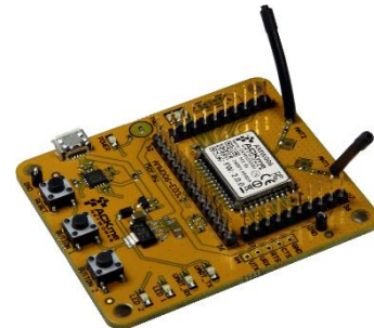
Figure 9 - AMW006-E03 eval board with wire antennas
