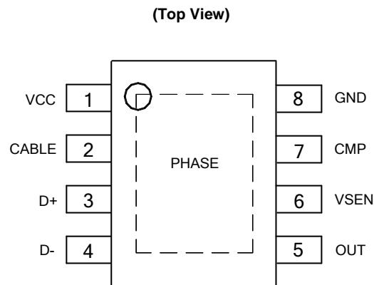
Note: The PHASE pin of BUCK converter is exposed PAD, which is at bottom of the IC (the dashed box).
