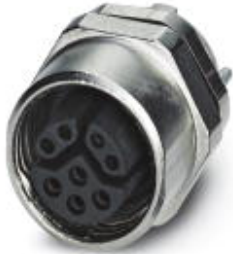
Hybrid flush-type socket, Ethernet, 8-pos., M12 SPEEDCON, rear/screw mounting with M12 thread, with straight solder connection
