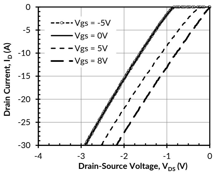
Figure 9. 3rd quadrant characteristics at  $T_J = -55^\circ\text{C}$
