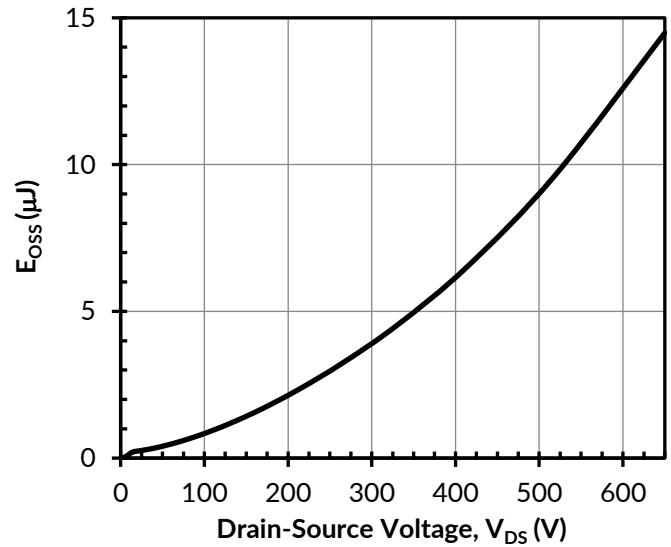
Figure 12. Typical stored energy in  $C_{\text{OSS}}$  at  $V_{\text{GS}} = 0\text{V}$
