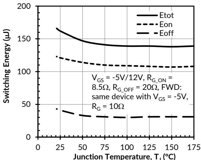
Figure 21. Clamped inductive switching energy vs. junction temperature at  $V_{DS} = 400V$  and  $I_D = 20A$
