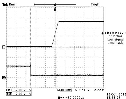
Figure 14. Startup from on/off
