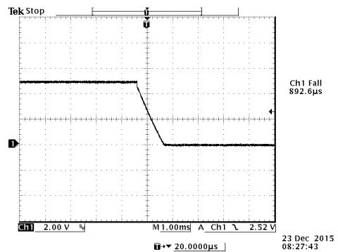
Figure 19. Vin=48V, Io=6A, Vo=5, with  $C_{ext}=1000\mu F$
