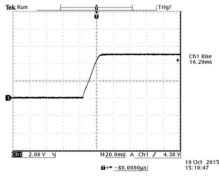
Figure 11.  $V_{in}=48V$ ,  $I_o=6A$ ,  $V_o=5$ , with  $C_{ext}=1000\mu F$
