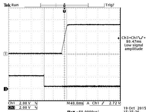
Figure 15. Startup from on/off
