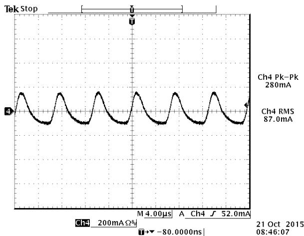
Figure 2. *is* (input reflected ripple current), AC component
