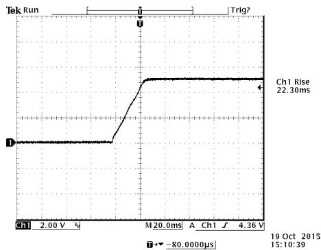
Figure 10.  $V_{in}=48V$ ,  $I_o=6A$ ,  $V_o=5$ , with  $C_{ext}=1000\mu F$
