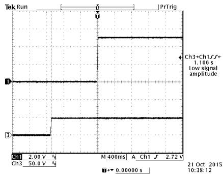
Figure 12. Startup from  $V_{in}$
