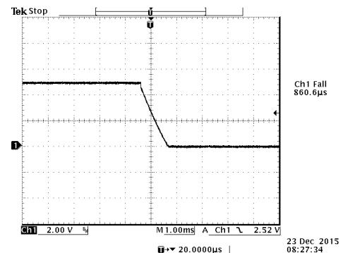
Figure 18. Vin=48V, Io=6A, Vo=5, with  $C_{ext}=1000\mu F$
