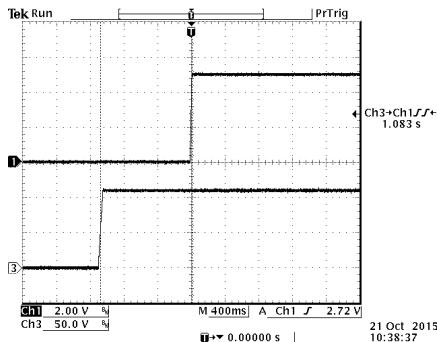
Figure 13. Startup from  $V_{in}$
