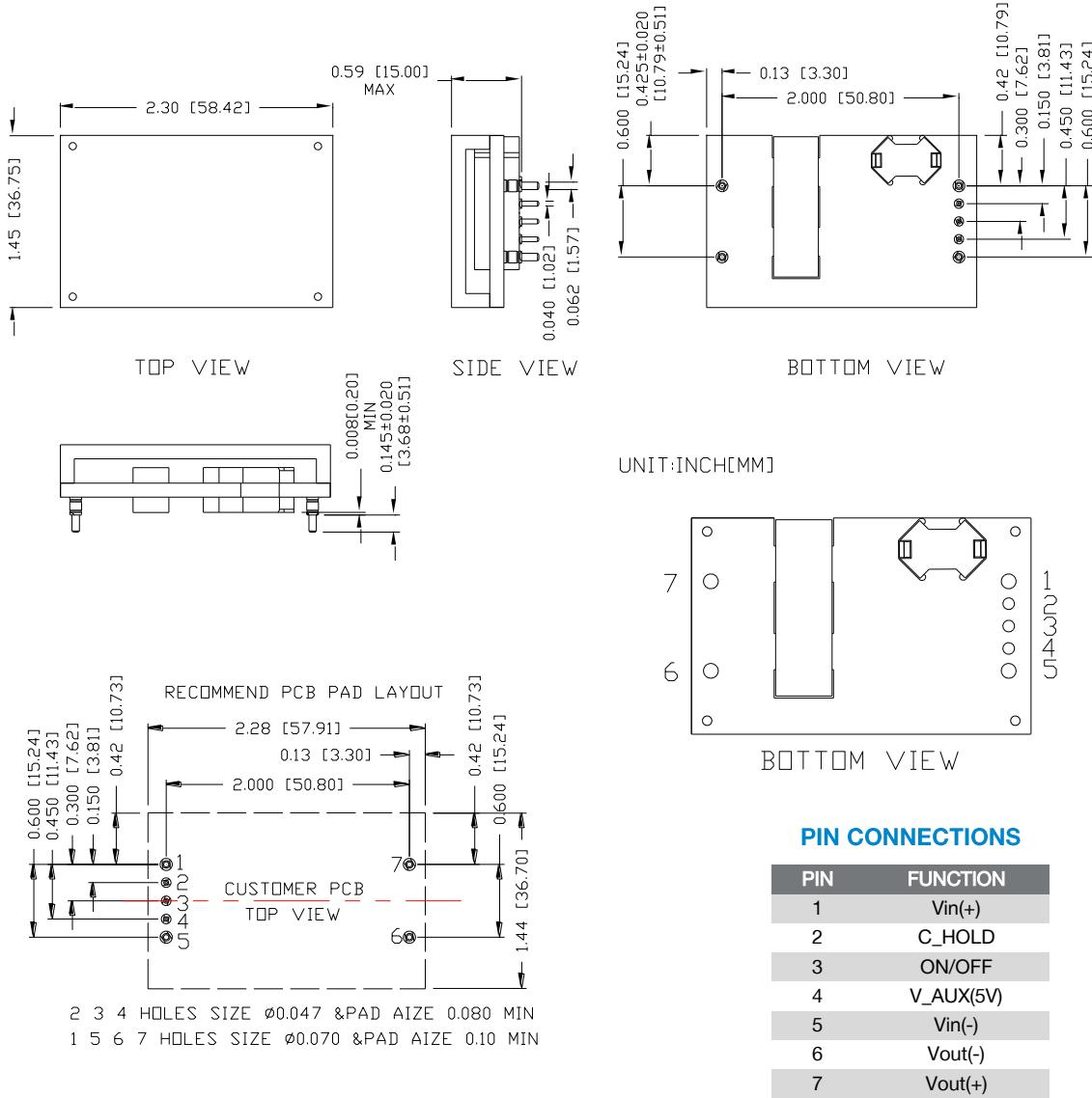
**NOTE:** This module is recommended and compatible with Pb-Free Wave Soldering and must be soldered using a peak solder temperature of no more than 260 °C for less than 5 seconds.
