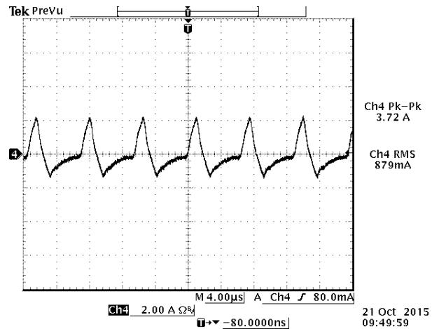
Figure 3. *ic* (input reflected ripple current), AC component
