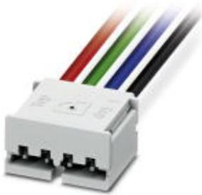
Plug component, Nominal current: 10 A, Rated voltage (III/2): 24 V, Number of positions: 4, Pitch: 1.9 mm, Color: white, Contact surface: Tin, Length of the punched-on cables: 500 mm for flexible PCBs with a width of 8 mm and a permissible PCB thickness in the contact zone of 0.15 mm ... 0.3 mm
