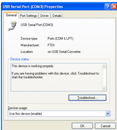
Figure 3-4 Access COM Port Properties
