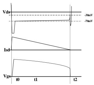
Figure 4—Synchronous Rectification
