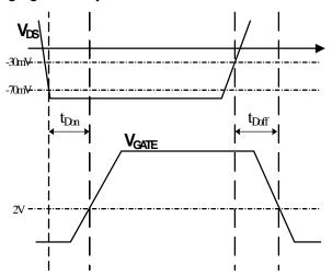
Figure 2—Turn on and Turn off delay
