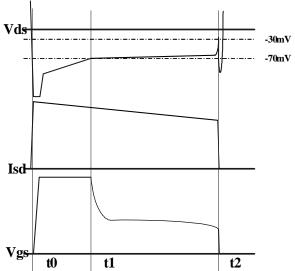
Figure 3—Synchronous Rectification Operation at heavy load
