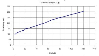
Figure 6—Total Turn-on Delay vs. Qg
