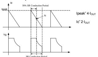
Figure 5—Synchronous Rectification typical waveforms in QR Flyback
