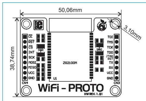
Figure 4: *WiFi-PROTO* board's dimensions
