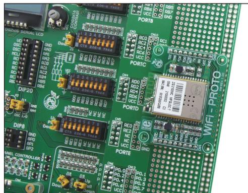
Figure 2: *WiFi-PROTO* soldered on the PROTO board
