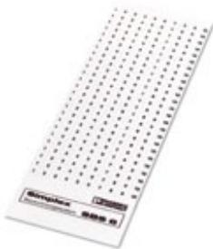
Marker for terminal blocks, Card, white, labeled, Printed horizontally: Consecutive numbers: Front 1 - 250, back 251 - 500, Mounting type: Snap into tall marker groove, Snap into flat marker groove, for terminal block width: 8.2 mm, Lettering field: 6 x 8.1 mm
