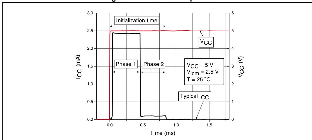
The initialization time is  $V_{CC}$  and temperature dependent. [Table 6](#) sums up the measurement results for different supply voltages and for temperatures varying from -40 °C to 125 °C.
