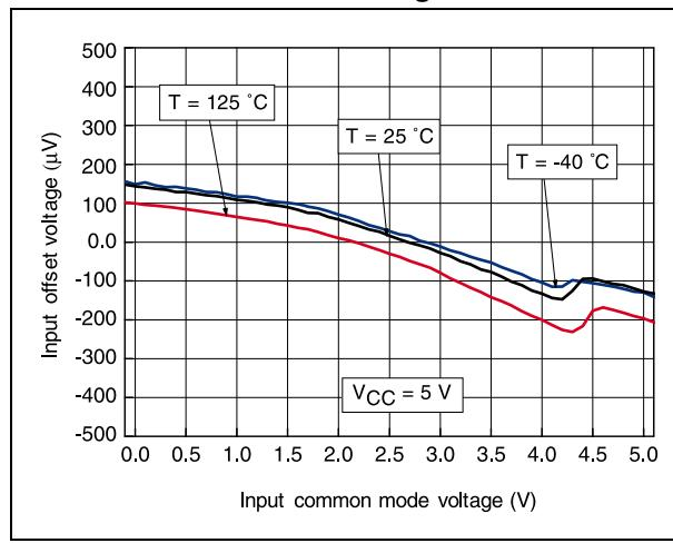
**Figure 7. Input offset voltage vs. temperature**
