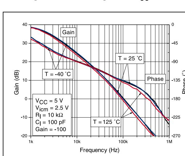
**Figure 13. Closed-loop gain diagram vs. capacitive load**
