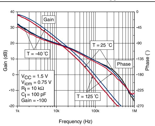
**Figure 12. Bode diagram at  $V_{CC} = 5 \text{ V}$**
