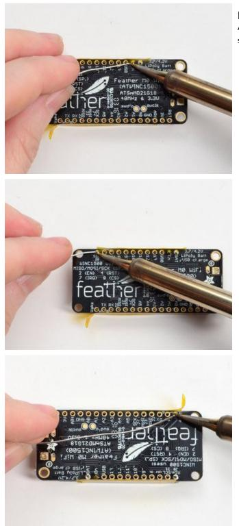
Flip & Tack Solder After flipping over, solder one or two points on each strip, to 'tack' the header in place
