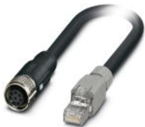
Bus system cable, VARAN, 6-pos., black halogen-free TPE, shielded, straight M12 SPEEDCON plug to RJ45 plug-in plug (IP20), cable length: 7 m
