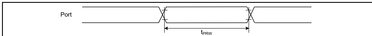
Figure 2.28 I/O ports input timing
