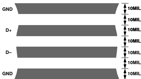
Figure 34. Arrangement of Signal Tracks
