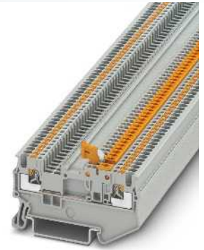
1.5 (1.5) mm 2 , 10 A, knife disconnect terminal block, two connections, bridgeable
