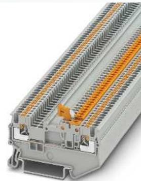
1.5 (1.5) mm 2 , 10 A, knife disconnect terminal block, two connections, bridgeable
