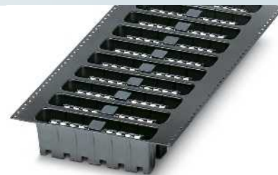
Pin length of 2.0 mm, taped PCB terminal blocks, connection direction vertical to the PCB
