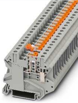
4 (6) mm 2 , 20 A, knife disconnect terminal block, with test socket screws
