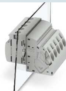
16 mm 2 panel feed-through terminal block, external part with push-in connection, internal part with screw connection
