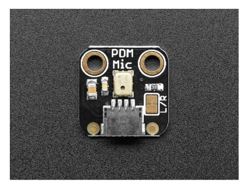
The 4-pin JST connector has **3V**, **GND**, **DAT**, **CLK** connections that can be used with one of our JST-SH cables to make a flexible mic arrangement (https://adafru.it/FGS). If you want a version with breakout headers, we have a version here (https://adafru.it/FB0). An on-board solder jumper lets you change the mic from Left to Right channel
