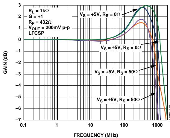
Figure 11. Small Signal Frequency Response vs. Supply Voltage
