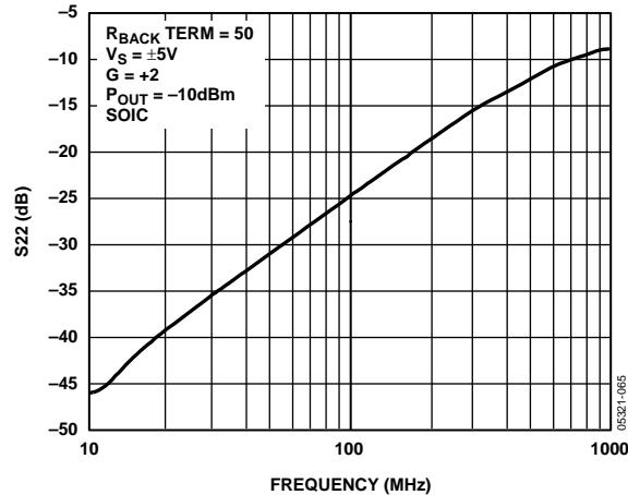
Figure 45. Output Voltage Standing Wave Ratio ( $S_{22}$ )
