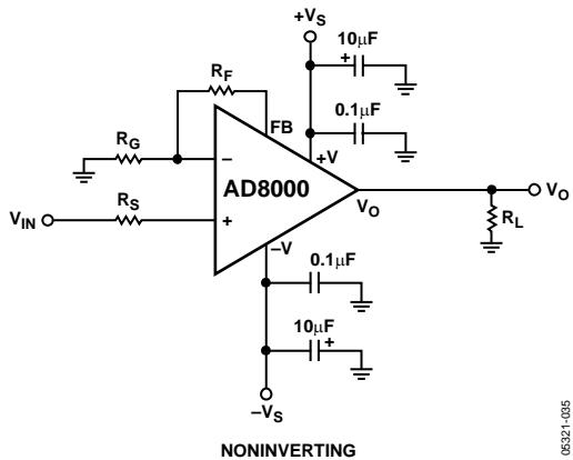
Figure 50. Noninverting Configuration
