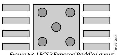
Figure 53. LFCSP Exposed Paddle Layout
