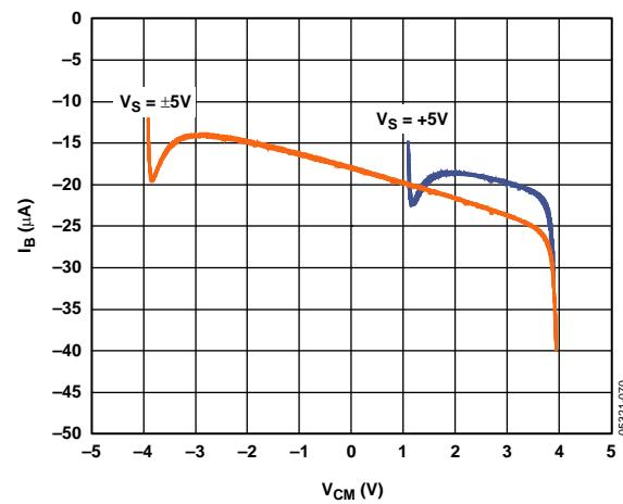
Figure 44. Input Bias Current vs. Common-Mode Voltage
