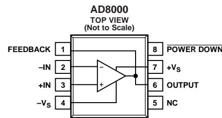
Figure 2. 8-Lead AD8000 SOIC\_N\_EP (RD-8-1)
