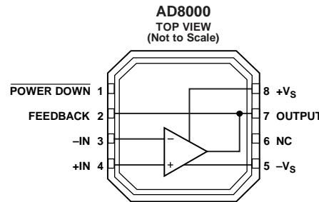
Figure 1. 8-Lead AD8000, 3 mm × 3 mm LFCSP\_VD (CP-8-2)
