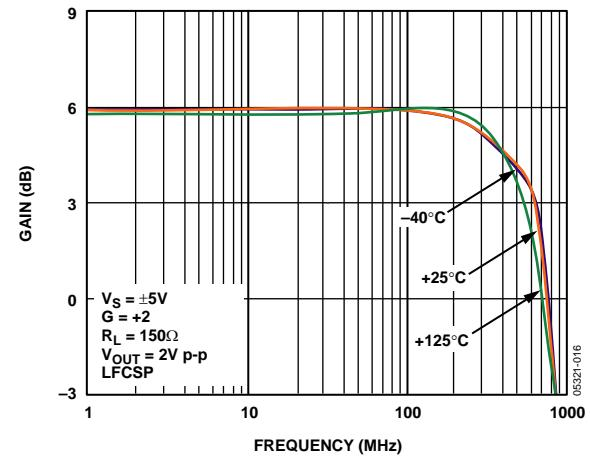
Figure 16. Large Signal Frequency Response vs. Temperature
