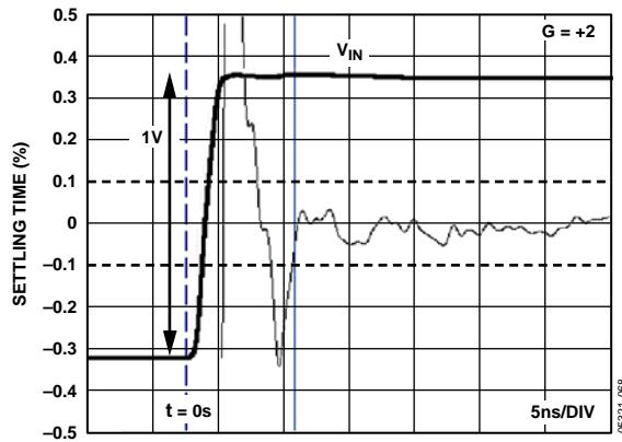
Figure 36. Settling Time
