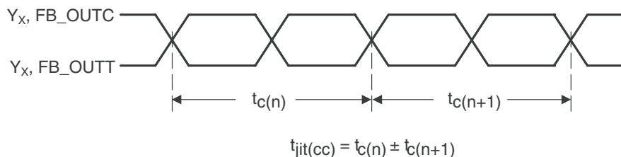
Figure 3. Cycle-to-Cycle Jitter
