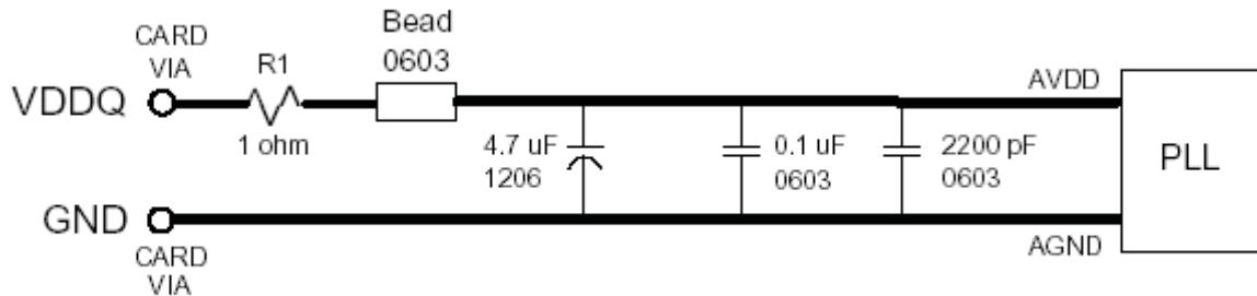
Figure 11. AV<sub>DD</sub> Filtering
