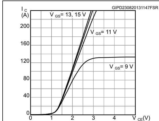
Figure 3. Output characteristics ( $T_J = 175^\circ\text{C}$ )
