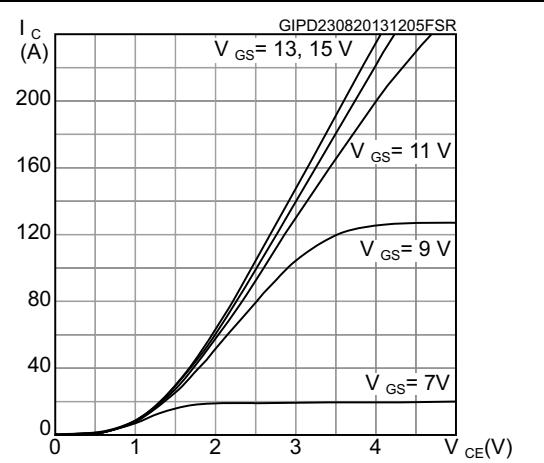
Figure 4. Transfer characteristics
