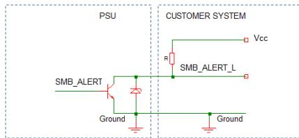
Figure 5. SMB\_ALERT\_L Connections
