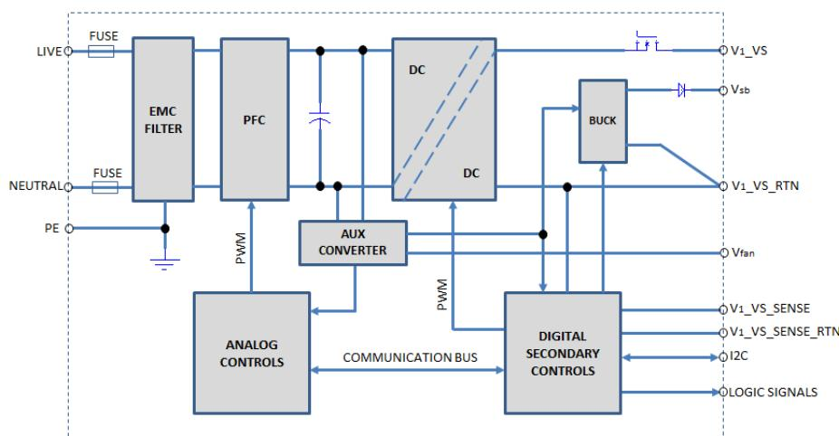
Figure 1. ABC600 SERIES Block Diagram
