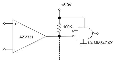
Figure 24. Driving CMOS/TTL
