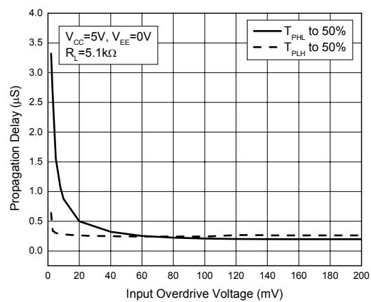
Figure 11. Propagation Delay vs. Input Overdrive Voltage
