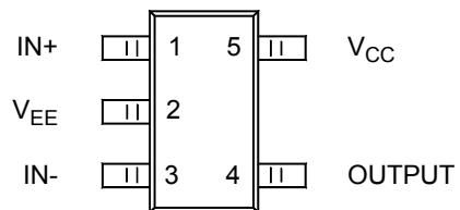
Figure 2. Pin Configuration of AZV331 (Top View)
