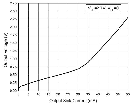
Figure 9. Output Voltage vs. Output Sink Current
