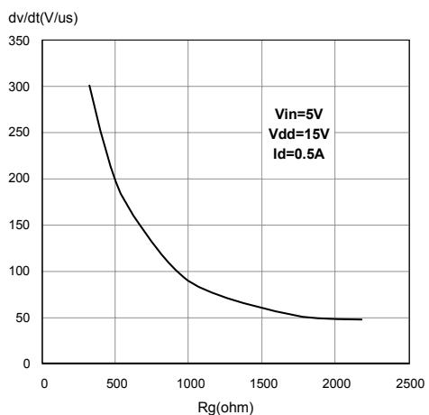
**Figure 21. Turn-off drain-source voltage slope (part 2/2)**
