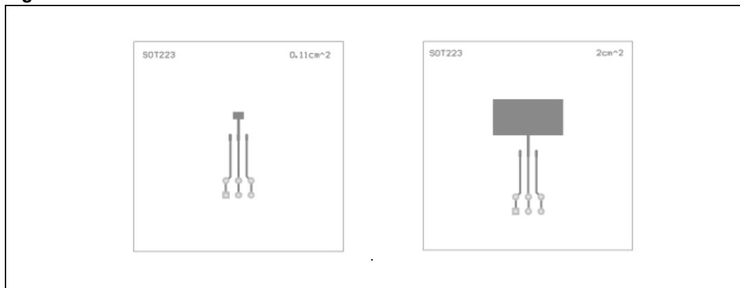
1. Layout condition of  $R_{th}$  and  $Z_{th}$  measurements (PCB FR4 area = 58 mm x 58 mm, PCB thickness = 2 mm, Cu thickness=35  $\mu$ m, Copper areas: from minimum pad layout to 0.8 cm<sup>2</sup>).
