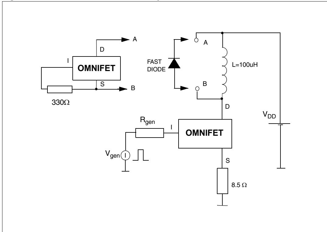
**Figure 6.** Unclamped inductive load test circuits
