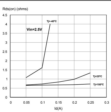
**Figure 12.** Static drain-source on resistance vs. input voltage (part 1/2)
