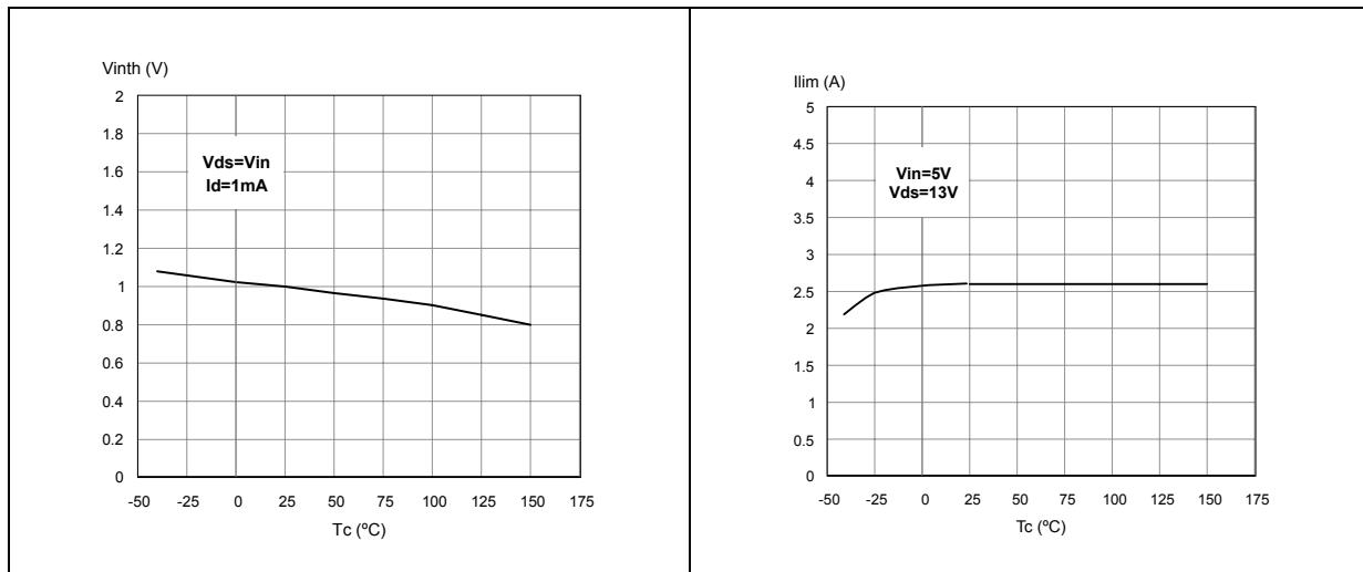
**Figure 28.** Normalized current limit vs. junction temperature
