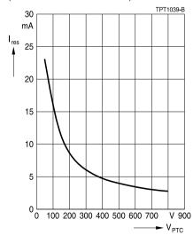
Minimum resistance of PTC thermistors versus applied voltage (pulsed)
