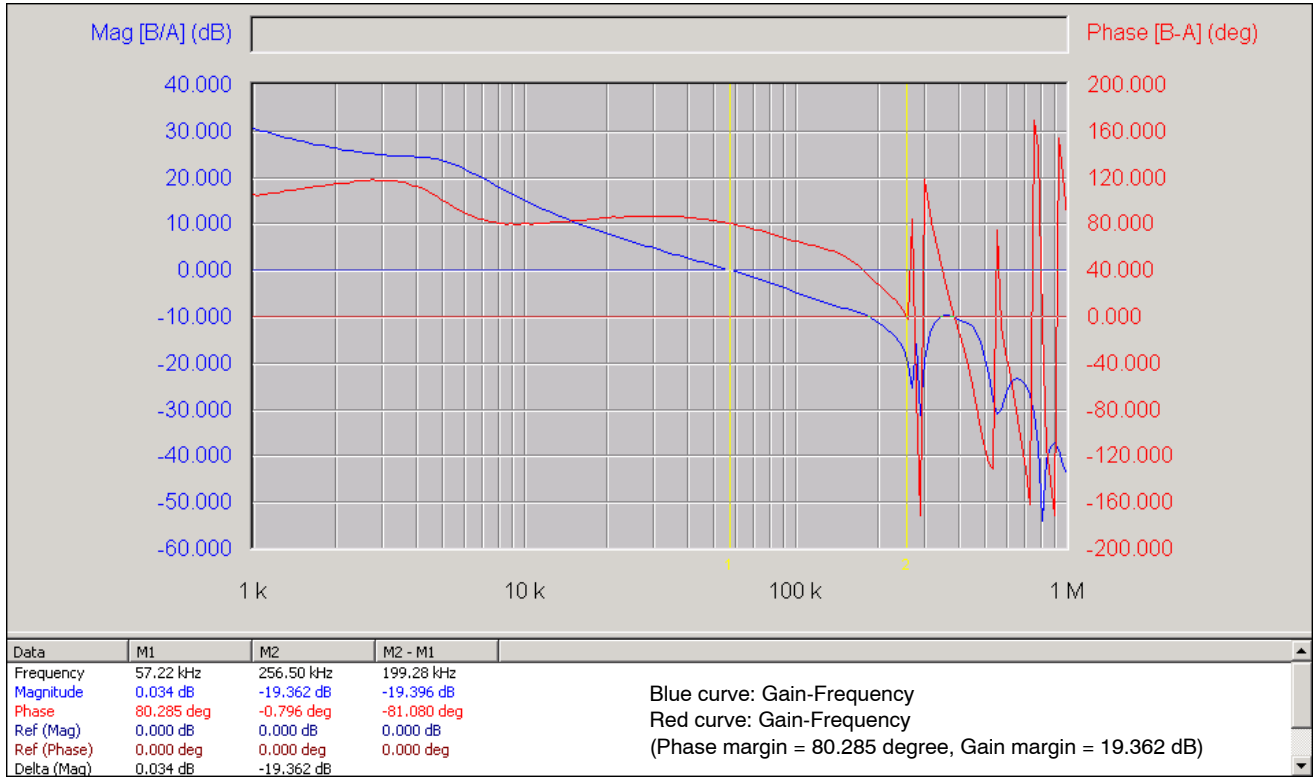
Figure 14. Closed-loop Voltage Loop-gain of the NCP1587
