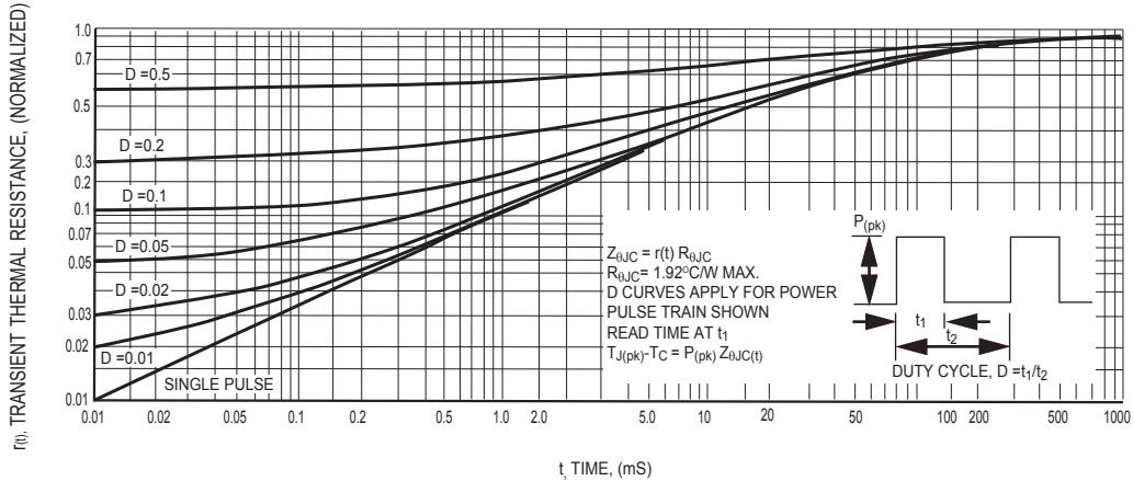
Figure 1 THERMAL RESISTANCE
