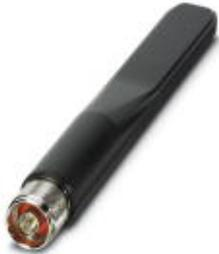
Omnidirectional antenna, 2.4 GHz/5 GHz, 2.5/5 dBi gain, linear vertical polarization, opening angle 2.4 GHz h/v 360°/30°, 5 GHz h/v 360°/16°, N (male), IP68; matching cable with panel feed-through Order No. 2701402
