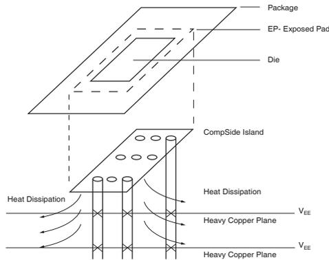
**PCB Thermal Consideration for 44-Pin QFN Package
