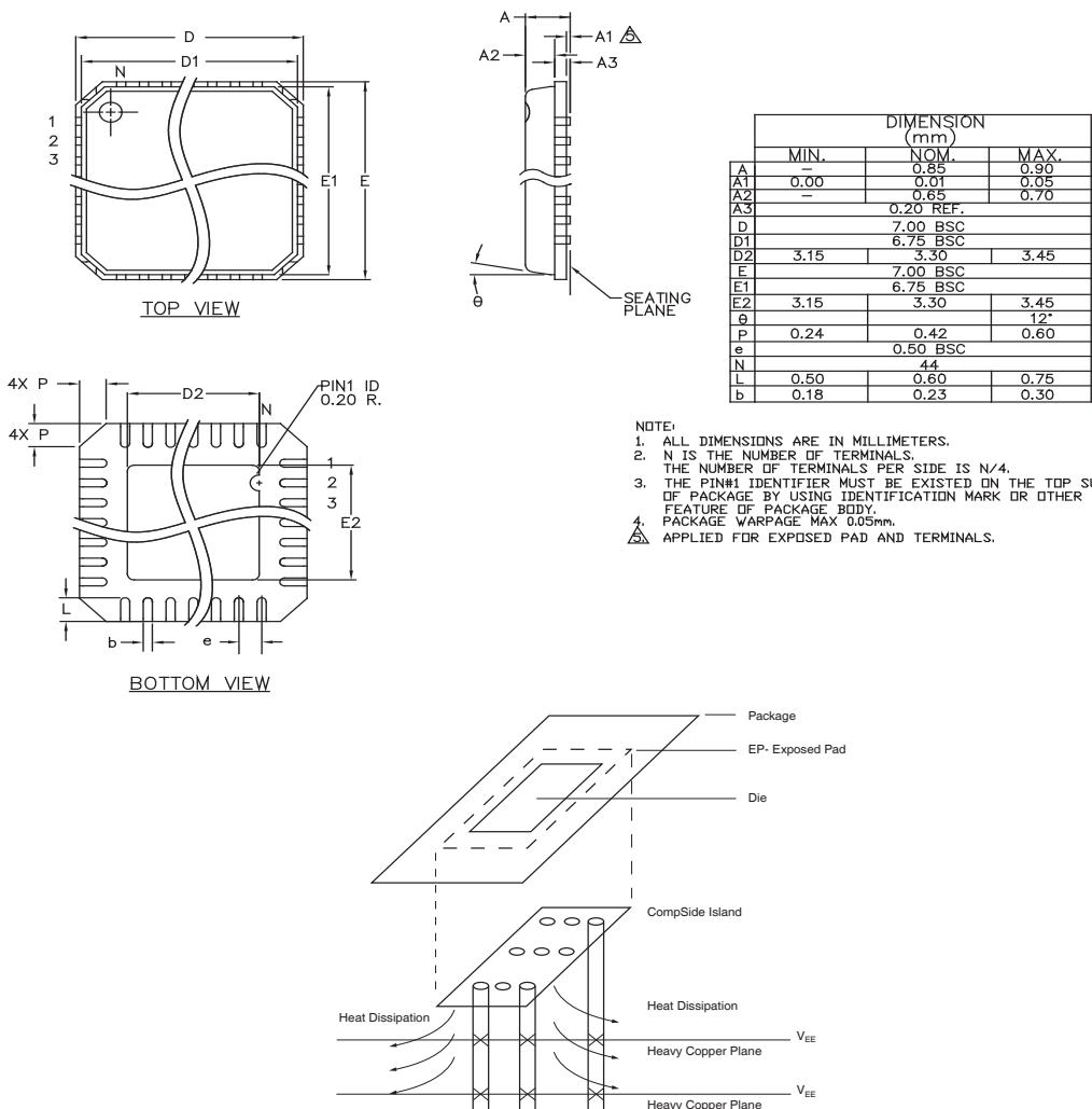
**PCB Thermal Consideration for 44-Pin QFN Package
