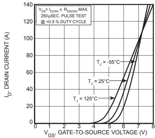
Figure 4, Transfer Characteristics
