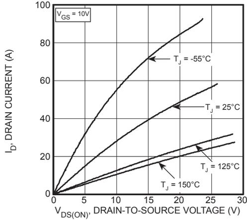
Figure 1, Output Characteristics
