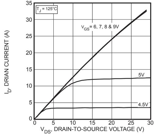
Figure 2, Output Characteristics
